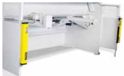
▶ Rear Protection Light Beams
