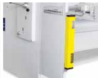
▶ Rear Protection Light Beams
